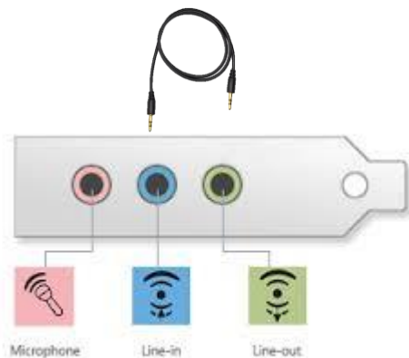
a. Line-out to Line-in direct connect, dual
