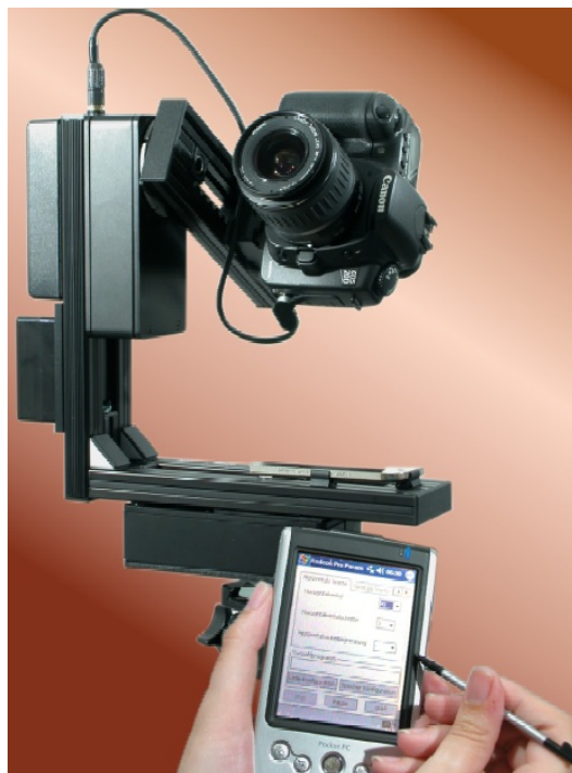
Figure 7.4: Automated panorama head. (Source: Wikipedia https://commons.wikimedia.org/wiki/File:Rodeon_vr_head_01.jpg )
