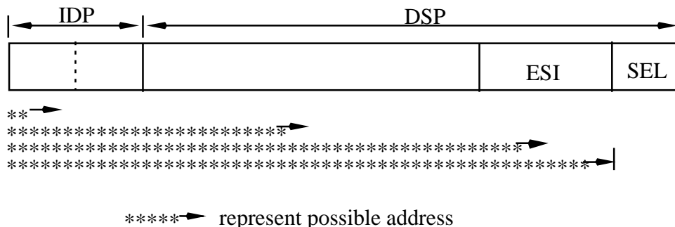
Figure 5-1: NSAP Address Structure and Address Prefixes
