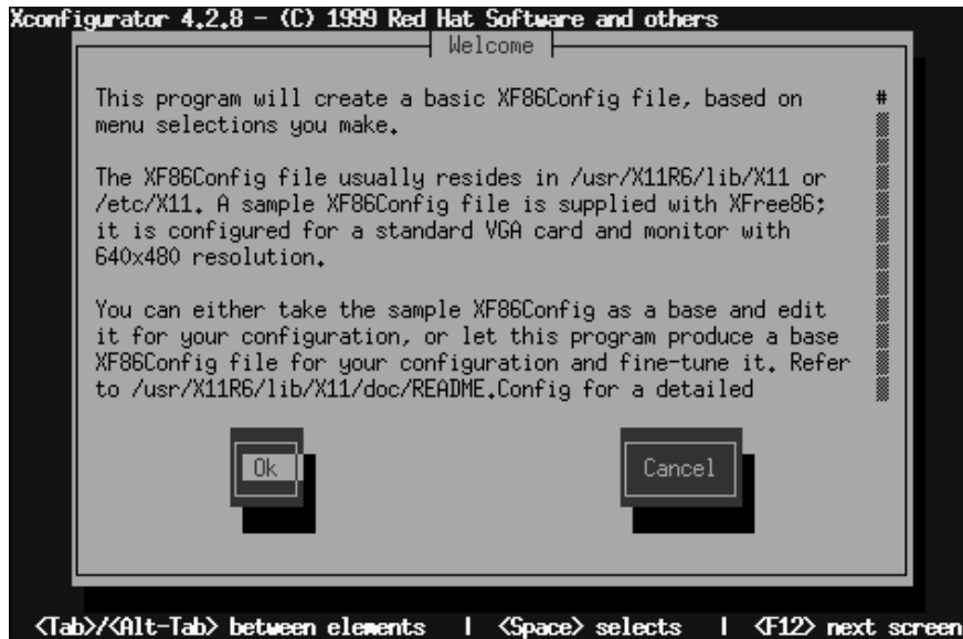
Figure 13–3 The Opening Dialog of XConfigurator
