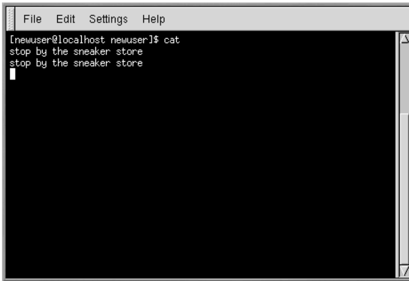
Figure 10–7 cat Demonstrates Standard Input and Standard Output
